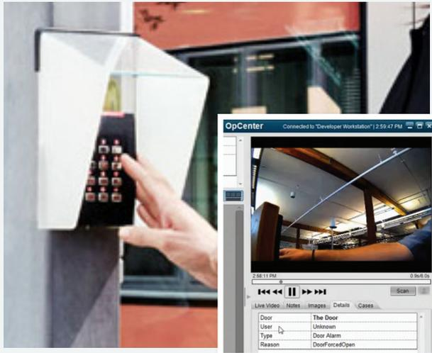
AXIS A1001 access control integrated with 3VR's Event Management provides event-driven video viewing and integrated alarm management by correlating live and recorded video with access control events.
